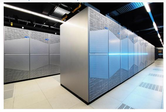
BullSequana, 3,000+ nodes, 370,000+ cores, AMD Milan, 14 PFLOPS 815 TB main memory, 130 PB disk storage, 60 GPU nodes (visualization, machine learning, faster codes) hot liquid cooling with high efficiency
